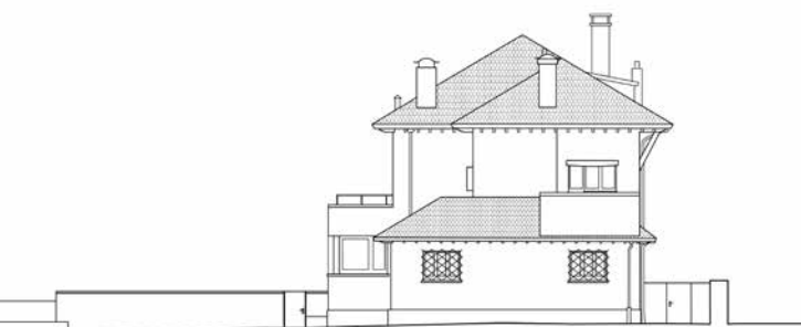
Facade views show the hipped roofs before the restoration.
